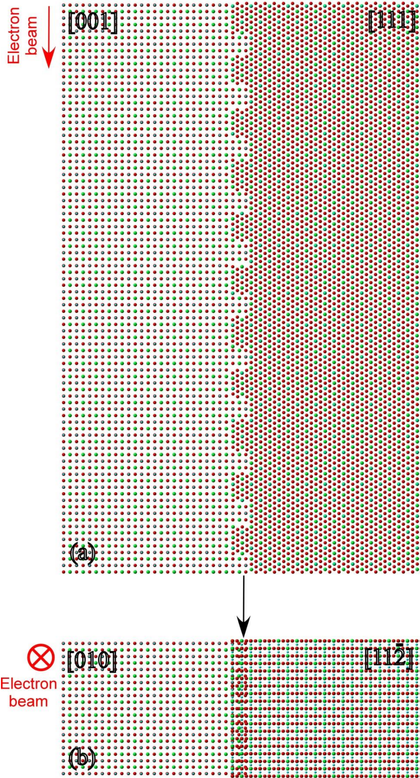
Figure 9: (a) Boundary model with 21 inclined steps. The grain on the left is oriented along [001] zone axis and the grain on the right is oriented along [111] zone axis. (b) The boundary after rotating (a) by 90^\circ to the orientation used to simulate the image in Figure 10. The
