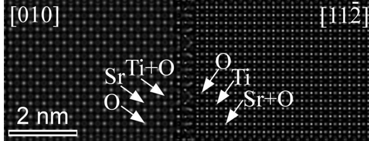
Figure 10: Simulated HRTEM image of an edge-on grain boundary (Figure 9b) under negative Cs imaging conditions with inclined steps ( C_s = -7\mu\text{m} , defocus = 4 nm, accelerating voltage of 300 kV). The left grain is oriented along [010] zone axis and the right grain along [11\bar{2}] zone axis.
